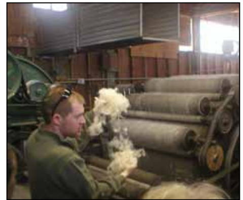
Yolo Wool Mill's carding equipment
